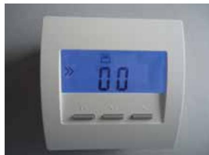
to uniquely identify the device within the bus system of a ZE central unit. You must only assign a device address once within the same RG/RS/RF device group and the same ZE. Within another device group (e.g. ST/SK/SF) or another ZE, you are allowed to reassign addresses and this can be sensible and sometimes even necessary.
