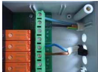
The power supply for the servomotors is connected to the top two terminals that are designated in the hatched field on the PCB as L for conductor and N for neutral. In the photo, two wires of a 4 x 1.5 mm<sup>2</sup> conductor are connected. This is the maximum cross-section that you can use. In most cases, it should however be over-dimensioned.
