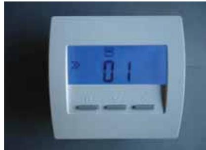
After this press the left-hand button once, the system address is displayed and you can see the programming symbol >> again on the left.
