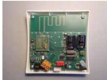
You can set this number using two jumpers at the bottom right-hand side of the PCB. When you do this, it is not important which device is given a particular number. You can also assign the only device on a ZE with any number you like between 1 and 4. The only important thing is that two devices on one ZE do not have the same number. This means that it does not matter how you insert the jumpers, they must only be inserted differently.
