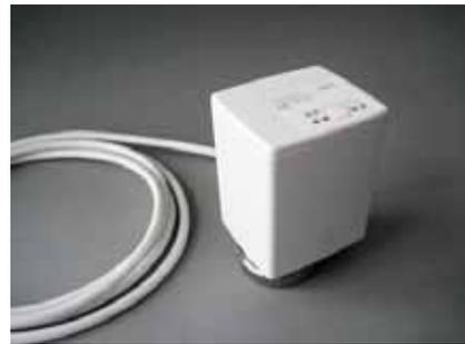
4. If the servomotor does not completely close the valve, a plunger extension can be installed (SF/SK 1 mm adapter). To do this, screw the servomotor off the valve and push on the extension cap preferably using a small pair of pliers. For this, the plunger has a small cam on the top side on which the cap is seated fairly tightly. Please ensure that you push the cap all the way on.
