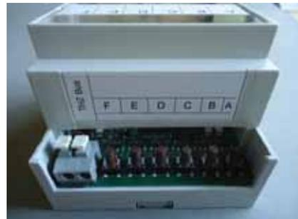
You can connect two solid state relays (SSRs) to each of the six outputs (but not more than eight SSRs in total). The SSRs must have a potential-free input (normally an optocoupler). The connection is normally made by means of a two-wire cable that must be wired with correct polarity. The polarity is stated on the housing.
