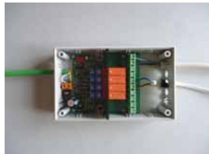
You connect the conductors of the consumers to the terminals for the individual relays. The connections for the four relays are designated A, B, C, D with a ~ symbol for the phase and an N for neutral. In the photo, the cable of a thermoelectric servomotor is connected. If necessary, you can implement tension relief with a cable tie as shown in the photo.
