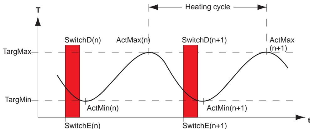
The cycle is run. The system registers deviations in the actual extreme values from the target extreme values and lead to changed parameters in the next cycle. In this way, information about the system and the environment is saved in the parameters. If these conditions change, the changes are reflected dynamically in changed parameters and lead to a changed control response.
