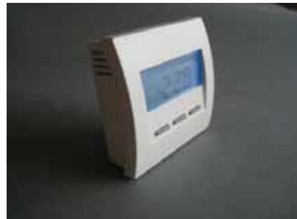
Power is supplied by two AA alkaline manganese batteries that you can access after removing the battery cover. The correct polarity is marked on the housing.
