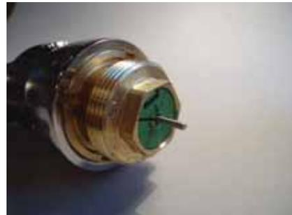
Check whether the servomotor is in the „open“ position. (The plunger must be retracted into the housing). This is very important. If you mount the servomotor in the „closed“ position, the plunger can jam such that the motor can no longer move it.
