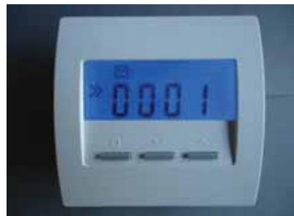
After this press the left-hand button once, the configuration is displayed and you can see the programming symbol >> again on the left. When doing this, you must ensure that you really press the left-hand button only once. The programming symbol must not flash. If the programming symbol does flash, you pressed the button more than once by mistake. You must then repeat the procedure.
