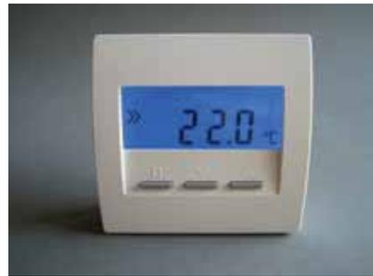
In modes Night/Off, the system additionally displays the Crescent Moon and X icons. It is not possible to display the associated target temperature, since the ZE cannot transfer it (see above).
