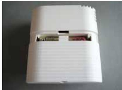
If the batteries run down, this is indicated by a battery icon on the display. Apart from this, the system sends an appropriate message to the ZE central unit that also displays a battery icon in the status menu to indicate that you need to change the batteries.
