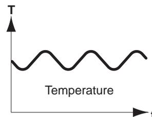
This yields the following approach (**Figure 2** in a much enlarged representation): A radiator is switched on for a specific time; the system responds to this a little later with a minimum and a maximum temperature.
