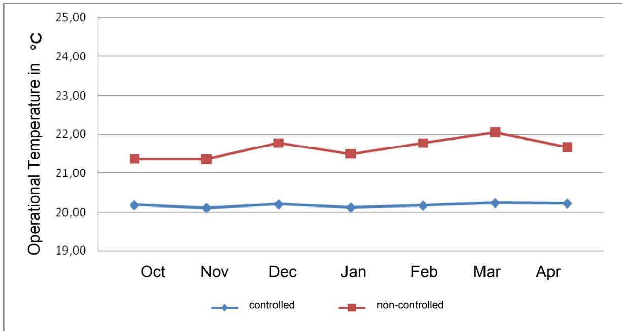
Figure 3.1. Monthly average values of operational room temperature in zones 1, 2, 5, 6, 8, 9, 11 (controlled / non-controlled option  $H_{vent} = 1.0$ ; intermittent operation)
