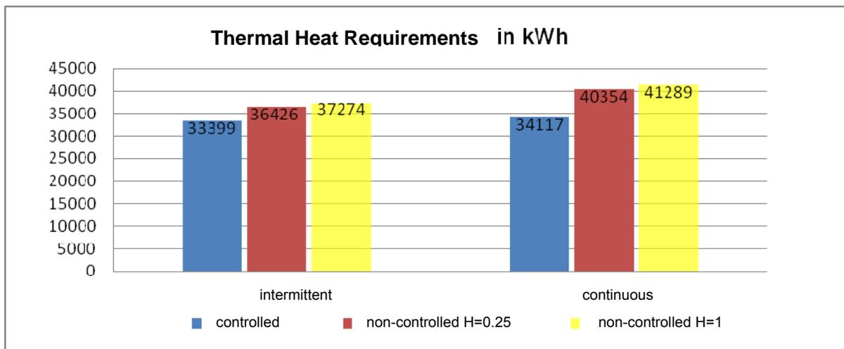
Figure 5.1 Thermal heat requirements in kWh/year under various operating conditions
