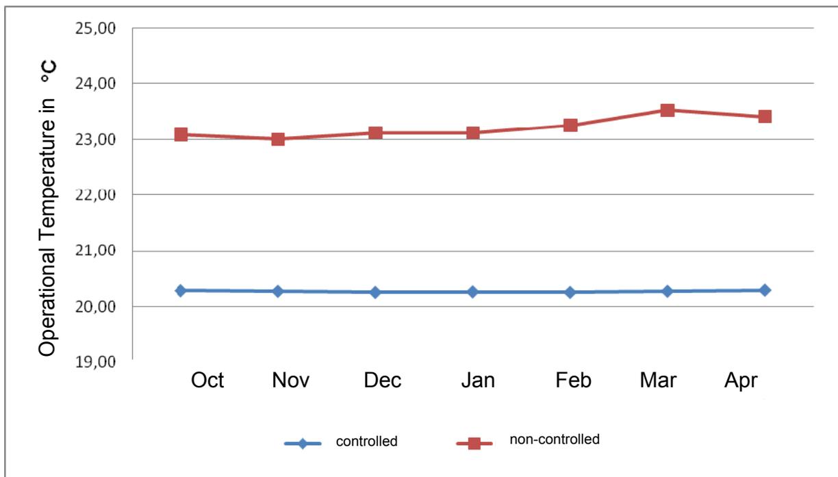
Figure 3.3. Monthly average values of operational room temperature in zones 1, 2, 5, 6, 8, 9, 11 (controlled / non-controlled option  $H_{vent} = 1.0$ ; continuous operation)
