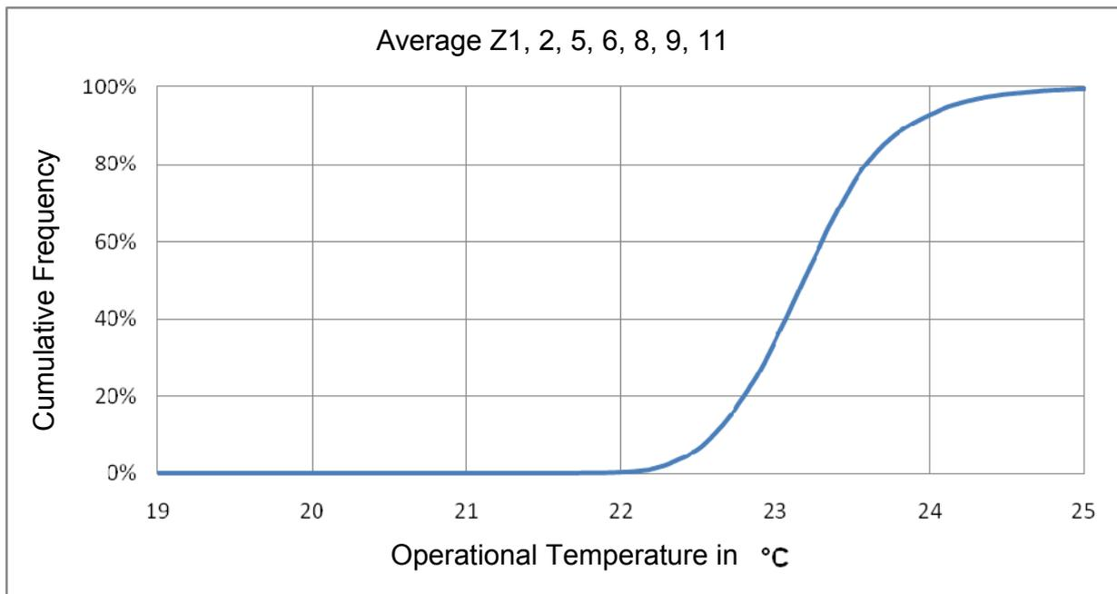
Figure 3.8. Cumulative frequency of room temperature (average value in zones 1, 2, 5, 6, 8, 9, 11; intermittent operation; non-controlled operation  $H_{vent} = 1; 0$ )
