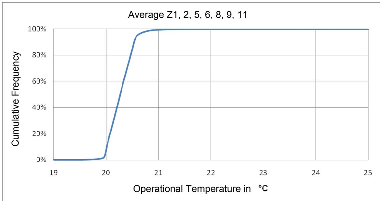
Figure 3.7. Cumulative frequency of room temperature (average value in zones 1, 2, 5, 6, 8, 9, 11; intermittent operation; controlled option)
