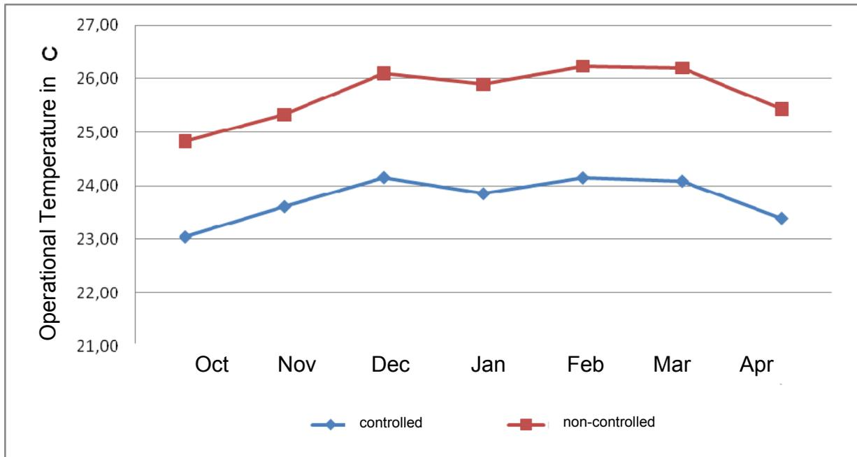
Figure 3.4. Monthly average values of operational room temperature in zone 10 (controlled / non-controlled option  $H_{vent} = 1.0$ ; continuous operation)
