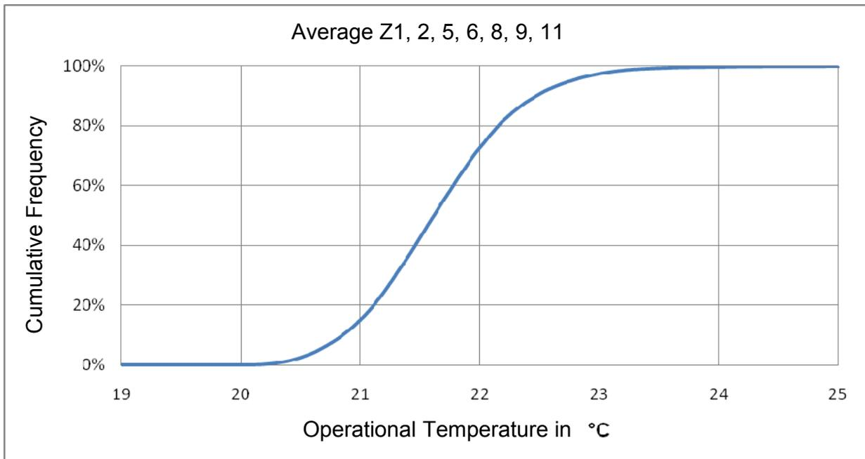
Figure 3.6. Cumulative Frequency of Room Temperature (Average Value in Zones 1, 2, 5, 6, 8, 9, 11; intermittierender Betrieb; non-controlled option  $H_{vent} = 1; 0$ )
