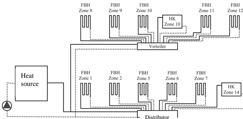
Figure 2.1. Star-shaped distribution for a mixed system with floor heating and free heating surfaces (basic principle)
