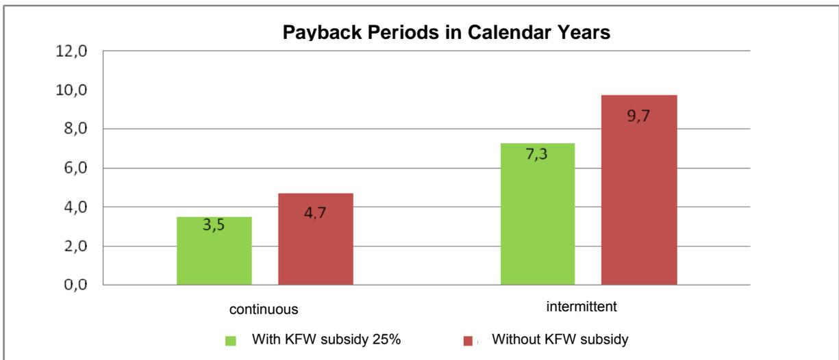
Figure 5.3 Payback periods for the retro-fitting with radio individual room controls
