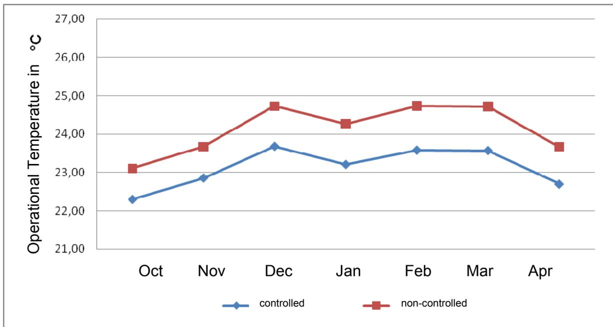
Figure 3.2. Monthly average values of operational room temperature in zone 10 (controlled / non-controlled option  $H_{vent} = 1.0$ ; intermittent operation)
