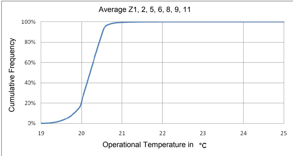
Figure 3.5. Cumulative Frequency of Room Temperature (Average Value in Zones 1, 2, 5, 6, 8, 9, 11; intermittent operation; controlled option)
